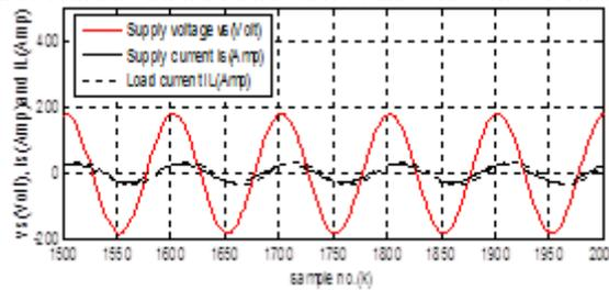
(a-2) The supply voltage, total supply current and load current signals after PFC.
