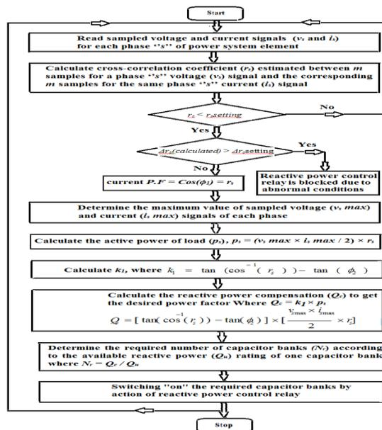
Fig. 1 Flow Chart for Reactive Power Control Relay Algorithm Based on Cross-Correlation Technique.
