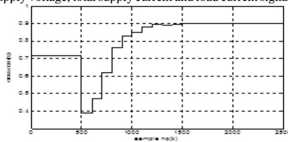
(b) Cross-correlation coefficient between phase voltage ( $v_s$ ) and current signal ( $i_s$ ).
