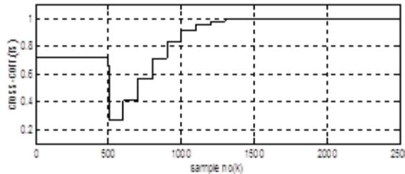
(b) Cross-correlation coefficient between phase voltage ( $v_s$ ) and current signal ( $i_s$ ).
