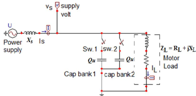
Fig. 2 The simulated circuit for power factor correction.
